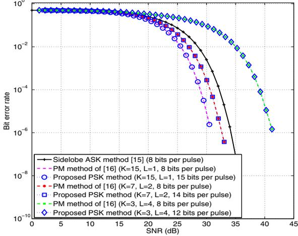
Fig. 3. BER versus SNR; second example.
