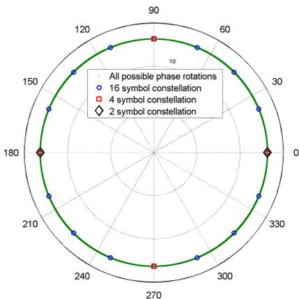
Fig. 2. Phase-rotation distribution versus spatial angle for a population of  $2^{12}$  and phase constellations for  $L = 1, 2,$  and  $4$ .
